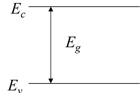
The diagram shows two horizontal lines representing energy levels. The top line is labeled  $E_c$  and the bottom line is labeled  $E_v$ . A vertical double-headed arrow between them is labeled  $E_g$ , representing the band gap.
