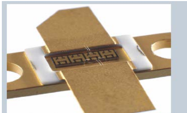
System-in-a-package assembly of AlGaIn/GaN HEMT power bar using a dedicated power package with direct heat sink.
