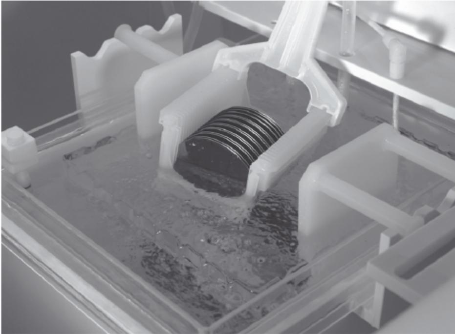
Figure 11.8 Wet etching tank. Courtesy VTT
