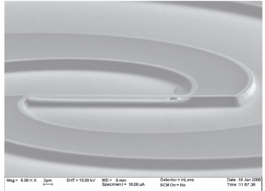
**Figure 11.16** Spiral antenna microbolometer: silicon is isotropically etched to release the narrow resistor. SEM courtesy Leif Grönberg, VTT
