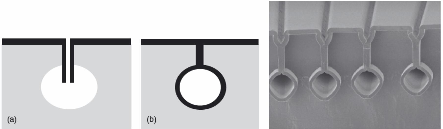
**Figure 21.15** Buried microchannels: (a) anisotropic DRIE, sidewall spacer formation and isotropic DRIE; (b) removal of spacer and conformal CVD. SEM micrograph from de Boer *et al.* (2000) by permission of IEEE
