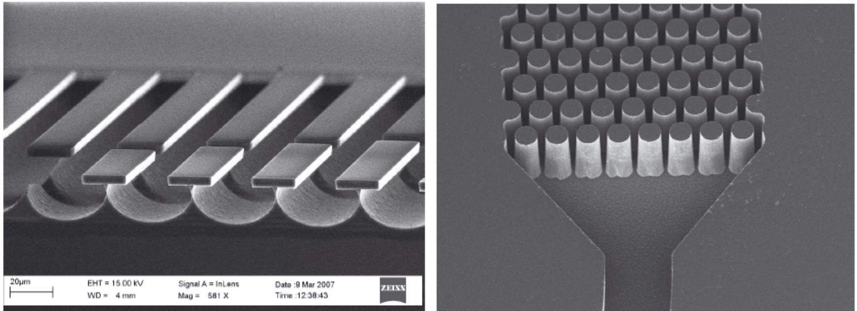
**Figure 11.4** Isotropic (left) and anisotropic etch profiles (right)
