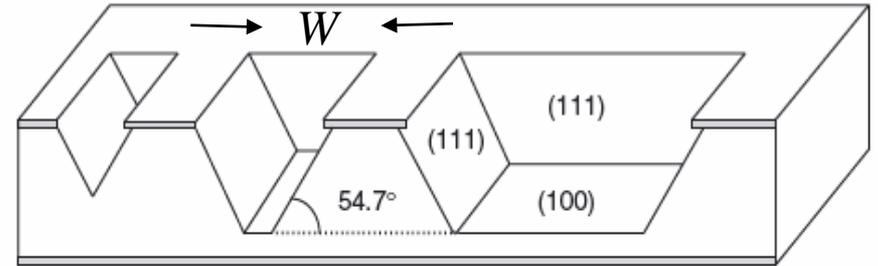
**Figure 20.1** Anisotropic wet-etched profiles in  $\langle 100 \rangle$  wafer. The sloped sidewalls are the slow etching (111) planes; the horizontal planes are (100). Etching will terminate if the slow etching (111) planes meet
