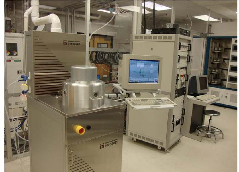
Combines physical ion milling with chemical etching.
