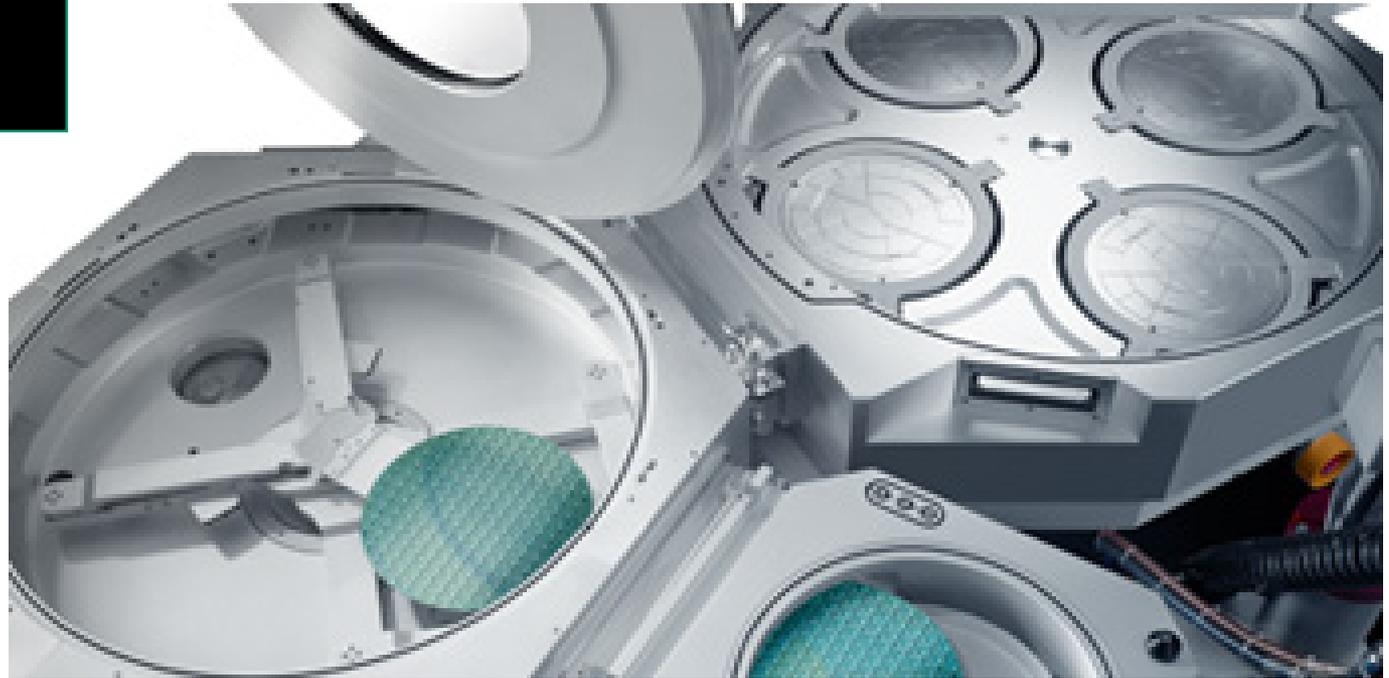
Lam's market-leading ALTUS systems combine CVD and ALD technologies to deposit the highly conformal films needed for advanced tungsten metallization applications. Nucleation layer formed using Lam's Pulsed Nucleation Layer (PNL) ALD process and in-situ bulk CVD fill.
