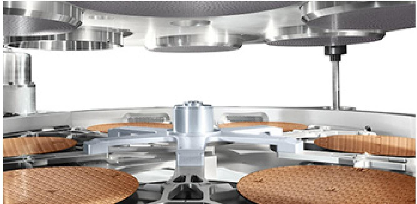
Strip processes remove photoresist material after it has served to “protect” certain areas of the wafer surface from being altered.
