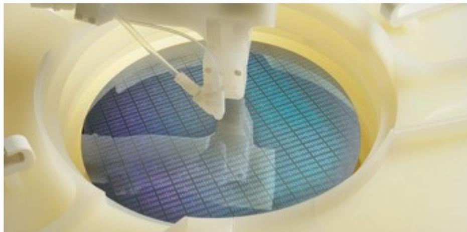
Wafer cleaning is a critical function that must be repeated many times during semiconductor manufacturing.
