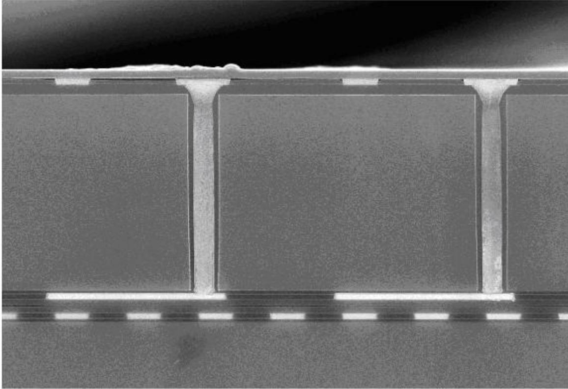
A vertical electrical connection (via) passing completely through a silicon wafer.
