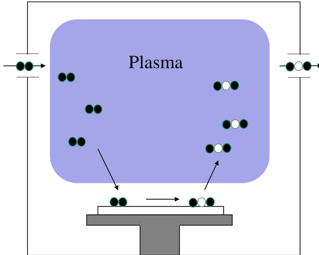
The plasma activates the etching gas which reacts at the surface to form a gaseous product.
