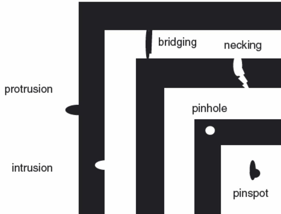
**Figure 8.10** Mask defects: extra chrome (protrusion, bridging, pinspot) and missing chrome (necking, intrusion and pinhole). If defect is very small, it may be cosmetic only because it does not print in lithography. Redrawn after ref. Skinner
