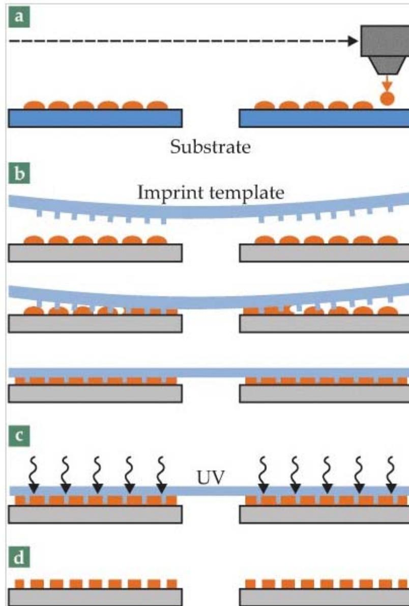
**Figure 3. Nanoimprint lithography**, the nanoscale version of a rubber stamp. After the liquid resist (orange) is dispensed onto the substrate **(a)**, the imprint template **(b)** mechanically molds it into the desired patterns. The resist is cured with UV light **(c)** to produce the nanoscale pattern **(d)**. (Adapted from ref. 18 .)
