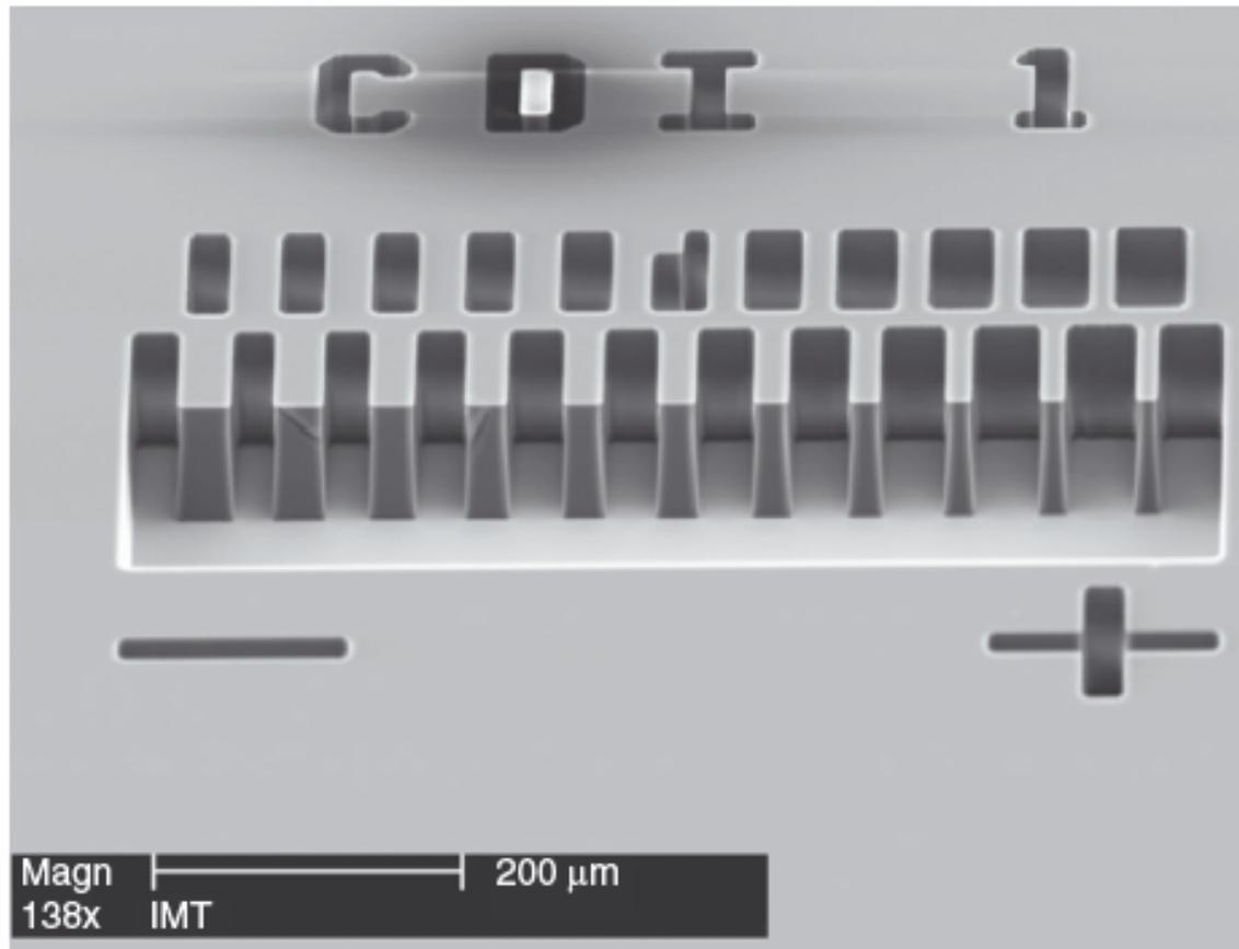
**Figure 9.6** Linewidth test structure of positive photoresist in SEM micrograph. Reproduced from Roth *et al.* (1999)
