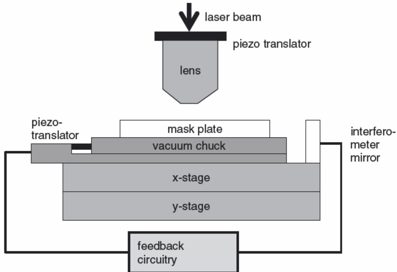
**Figure 8.7** Mechanics of the laser mask writer stage
