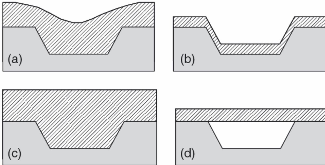
**Figure 9.8** Resist over topography: (a) spin coated; (b) spray coated; (c) cast; (d) laminated dry film
