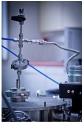
Gas inlet to the shower-head electrode
