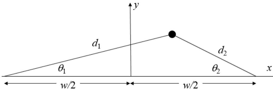
The equilibrium position for the mass is in the middle of the table ( $x = 0, y = 0$ ) where the forces exerted by the springs cancel each other out. If the mass is moved away from its equilibrium position then the force on the mass is,
