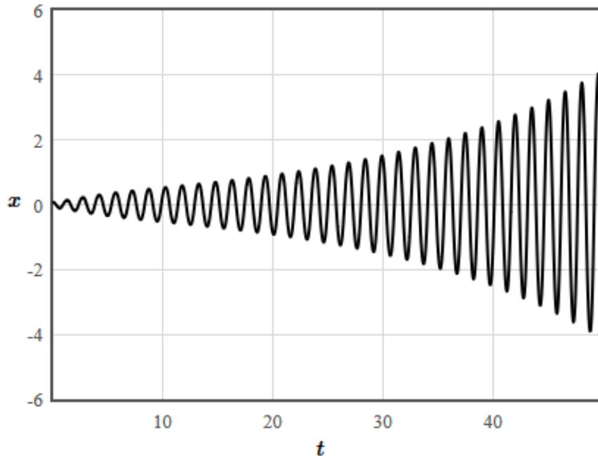
$$m \frac{d^2 x}{dt^2} + b \frac{dx}{dt} + \frac{mg}{l(1 - A \cos(\omega t))} x = 0.$$
