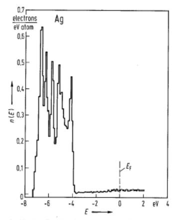
Fig. 15. Ag. Density of states calculated from the energy bands in Fig. 10. Ag [75Fon].
