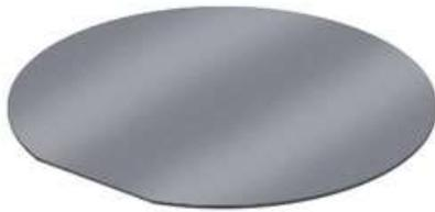
MOSFETs are made on {100} wafers
