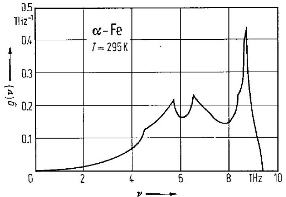
Fig. 3. Fe. Frequency spectrum of  $\alpha$ -iron at 295 K calculated from the Born-von Karman force constants of Table 3 Fe [67Mi1].
