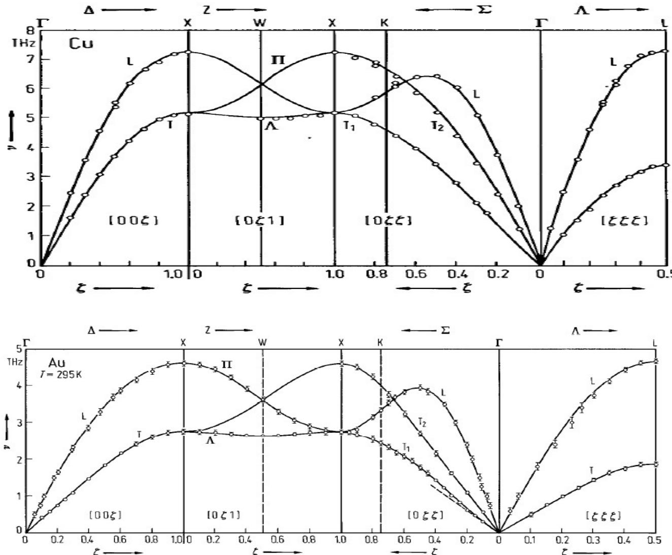
Fig. 1. Au. Phonon dispersion relations in the principal symmetry directions according to [73Ly1]. The solid curves represent both the fourth neighbour general force model (M1) and the fifth neighbour axially symmetric model (M2) of Table 3 Au. The dotted line in the  $\Sigma$  direction is corresponding to the velocity of sound appropriate to the  $[0\xi\xi]$  T<sub>1</sub> branch.
