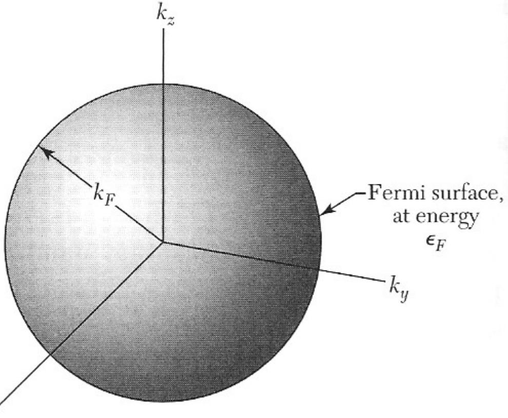
The thermal and electronic properties depend on the states at the Fermi surface.
