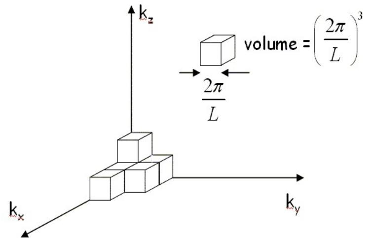
$$k_x, k_y, k_z = \dots, \frac{-4\pi}{L}, \frac{-2\pi}{L}, 0, \frac{2\pi}{L}, \frac{4\pi}{L}, \dots$$
