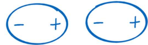
The dipole induces a dipole on the other atom.
