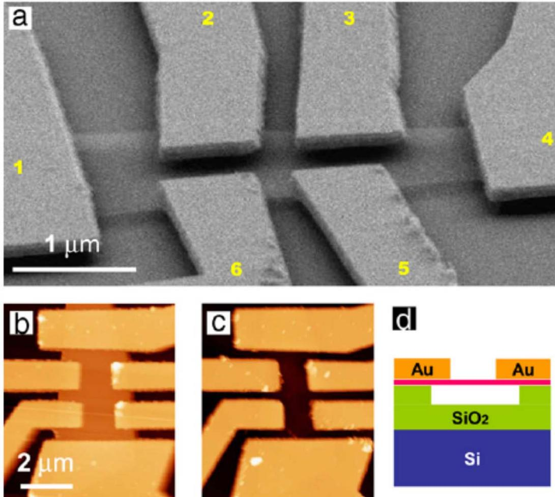
Mobility:  $200000\ \text{cm}^2/\text{V s}$  suspended,  $\sim 20000\ \text{cm}^2/\text{V s}$  otherwise
