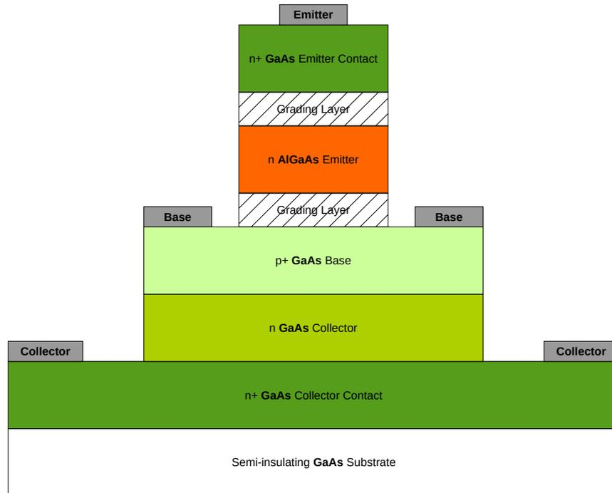
Figure 1: Structure of a NPN AlGaAs/GaAs HBT
