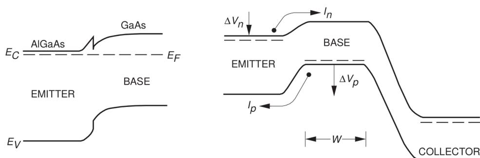
Figure 2: Band diagram of a AlGaAs/GaAs HBT: abrupt emitter–base junction on the left and a graded emitter–base junction on the right (2)
